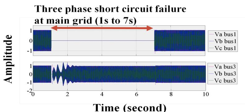
Local generator switched on after microgrid islanding, controlled by ultra-fast network
