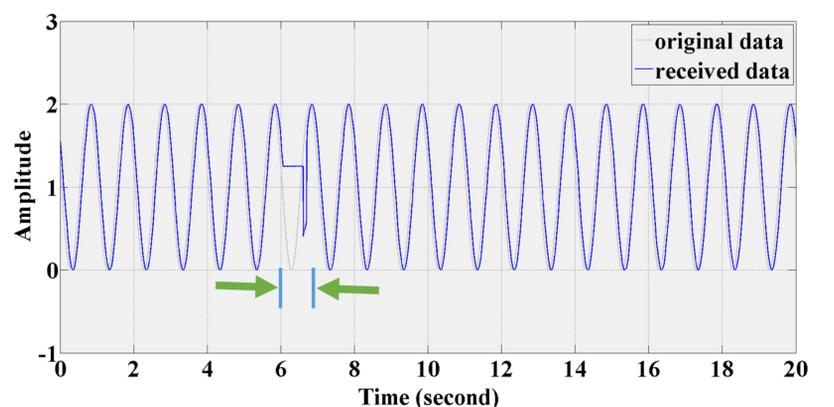
SDN controlled network path reconfiguration after link failure
