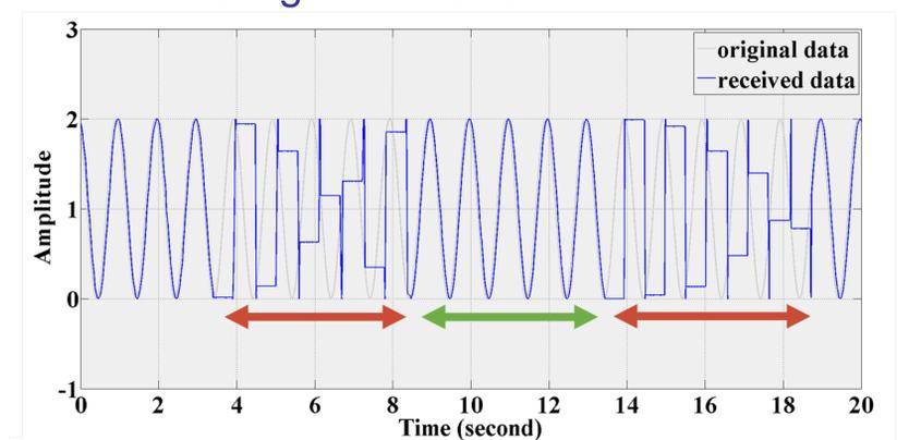
SDN controlled rate limitation (marked as red) for non-critical traffic
